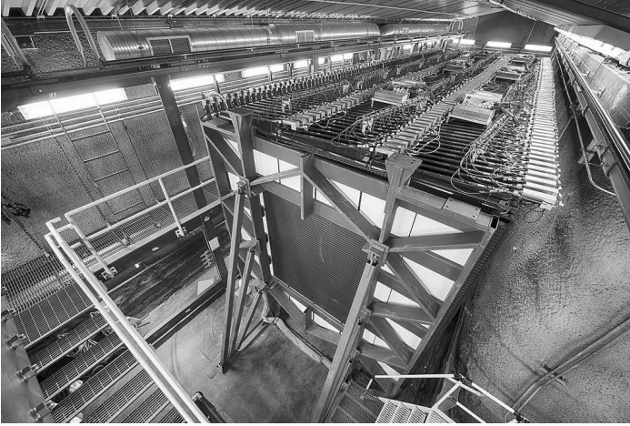
Figure 4.7. Top view of a part of the NOVA far detector with the neutrino beam produced at Fermilab in a distance of 810 km away (from [Fer19]). With kind permission from Fermilab.
